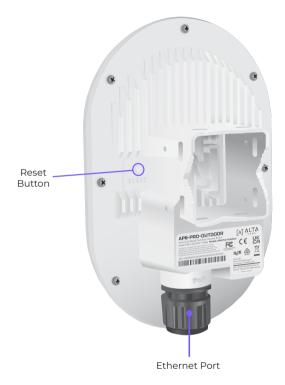
**Reset Button** Press down for 10 seconds until the LED begins flashing to reset the AP to factory defaults.
